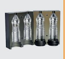
BLOW MOULD - RSBM / RE-HEAT STRETCH BLOWING
